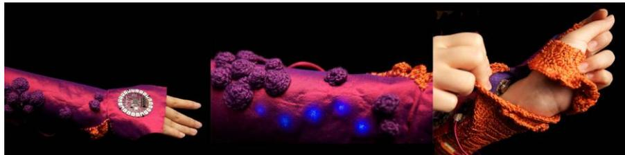
**Figure 4: soft-circuit armband design incorporating conductive yarn, LEDs, vibration and arduino lilypad and xbee**
