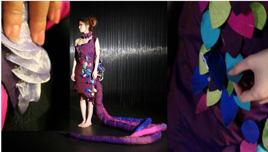
**Figure 3. *tendrils* stroke-sensor is hand-sewn using conductive silk organza and a row of resistors to enable positional tactile data to be sensed directly on the garment and actuated through the petals and motors**
